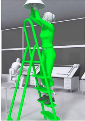
✓ Figure 5 Example where two hands need to be free for a brief period for light work. Keep two feet on the same step and the body (knees or chest) supported by the stepladder to maintain three points of contact. Make sure a safe handhold is available
